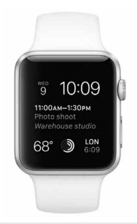
**Figure 3.** Wrist-mounted displays such as the Apple Watch (Apple, Cupertino, CA) may present other issues due to the limited screen area (approximately  $3.3 \times 4.2$ cm).
